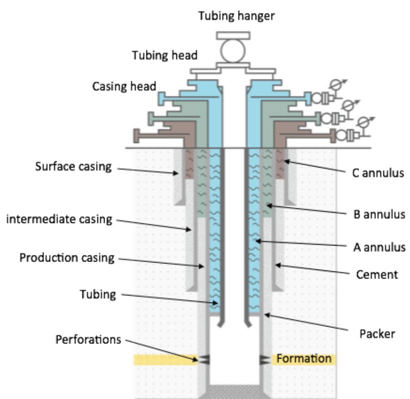
**Fig. 1.** Key elements of Well completion.
