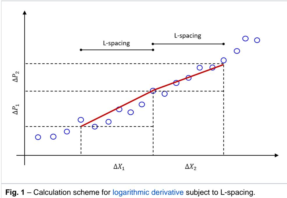
**Fig. 1 – Calculation scheme for logarithmic derivative subject to L-spacing.**
