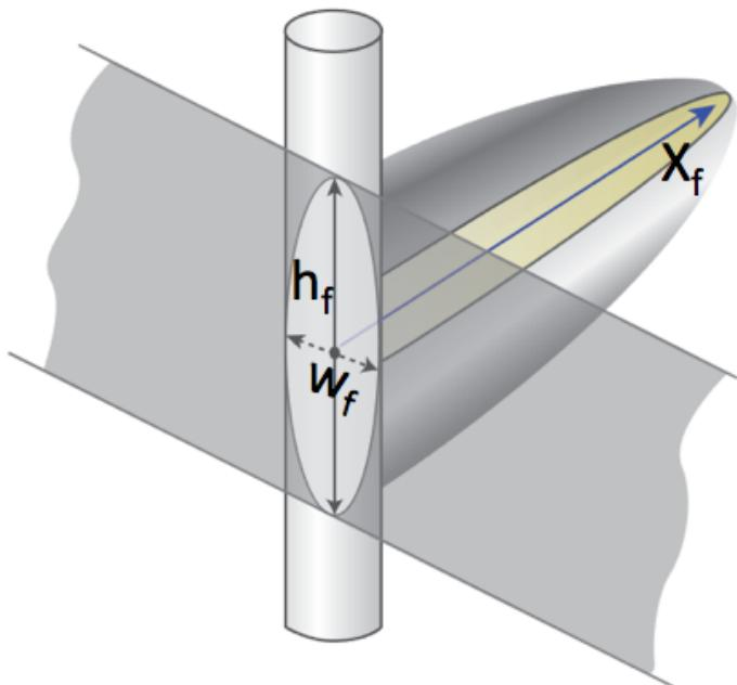
**Fig. 1 – Hydraulic fracture schematic showing fracture half-length ( $X_f$ ), fracture height ( $h_f$ ) and fracture width ( $w_f$ ).**
