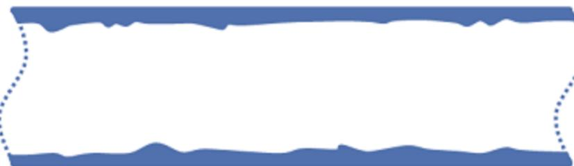
**Fig. 1.** Schematic view of inner wall pipe roughness
