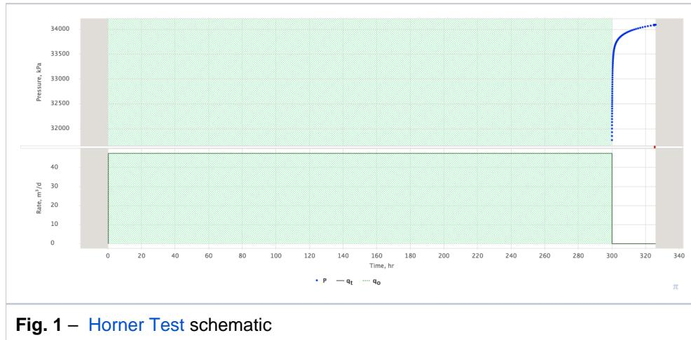
**Fig. 1 – Horner Test schematic**
