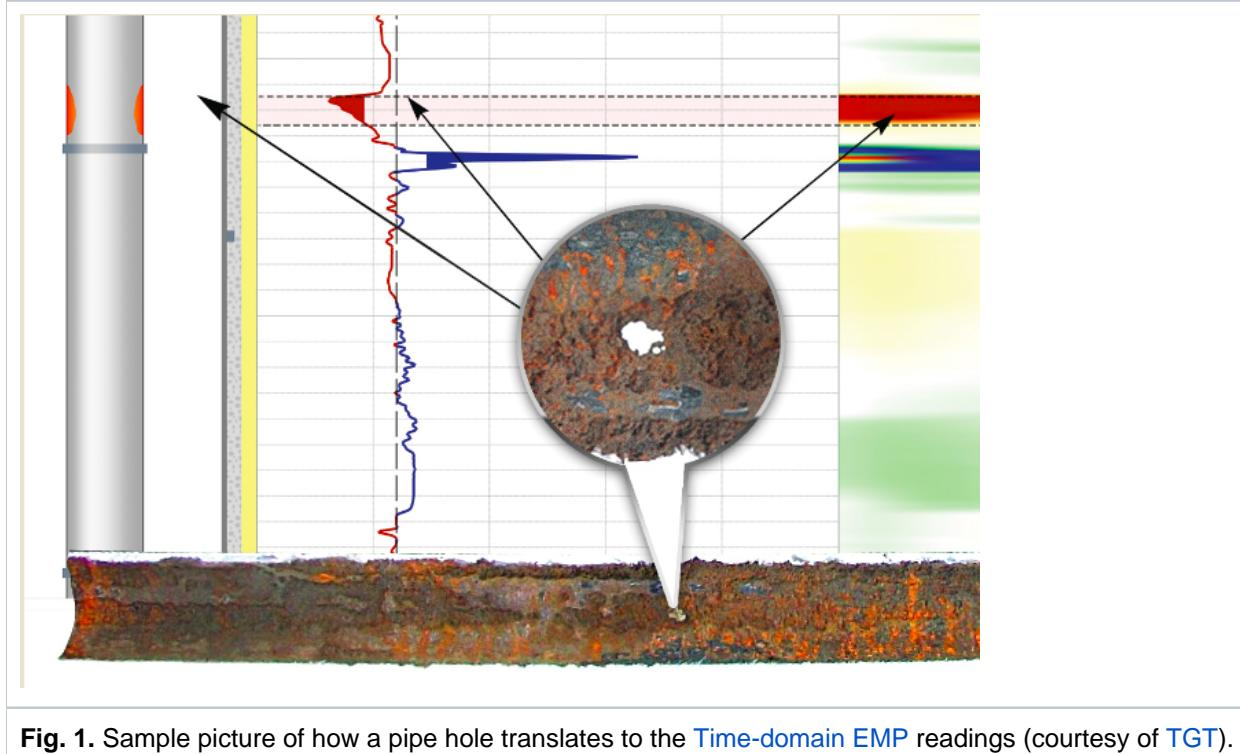
Fig. 1. Sample picture of how a pipe hole translates to the Time-domain EMP readings (courtesy of TGT).
